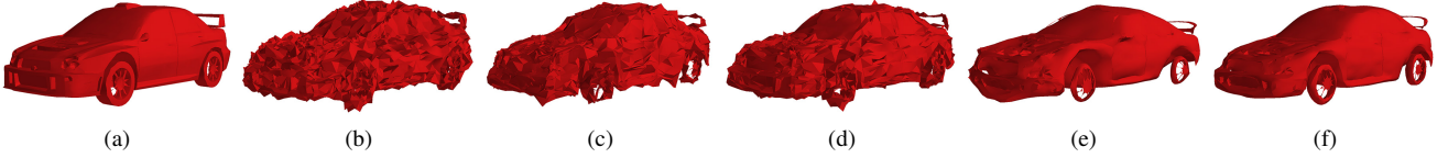
Fig. 6: Comparison of DMD-Net and CNR[54] trained on both ShapeNet and CNR dataset. (a) Ground truth, (b) Noisy Input, Output of (c) CNR network trained on CNR dataset, (d) CNR network trained on ShapeNet, (e) DMD-Net trained on CNR dataset, and (f) DMD-Net trained on ShapeNet.
